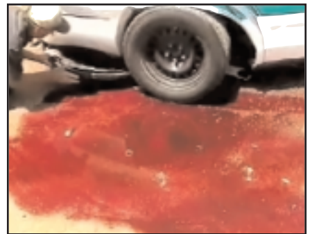
Post test shows massive tank leak
